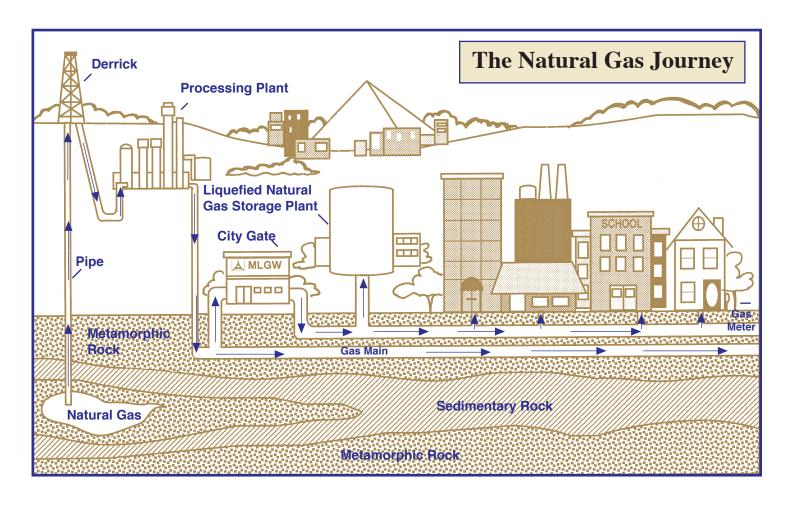
**Liquefied natural gas (LNG)** – A liquid form of natural gas obtained by chilling vapor gas to 259 degrees below zero. MLGW uses LNG to meet demand during peak periods.
