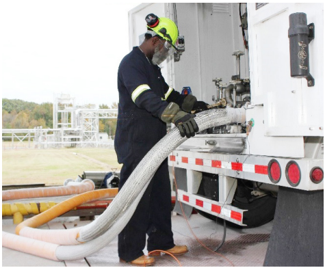
Tony McGuire with Kenan Advantage Group checks the connections on the vapor recovery hose and the LNG supply hose on his tanker at MLGW’s Capleville plant. The company provides LNG to United Parcel Service.
